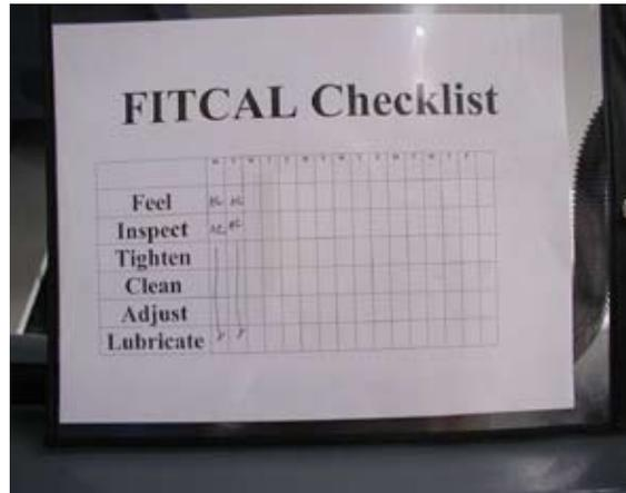
**A FITCAL checklist (shown above) records the six key preventive maintenance operations every grinding shop should perform: FEEL, INSPECT, TIGHTEN, CLEAN, ADJUST, LUBRICATE**
