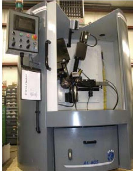
the parts used in grinding machinery require routine preventive maintenance and careful handling. Hit-or-miss maintenance techniques don't work. Specific instructions are needed. The easiest way to assure preventative maintenance is happening in your grinding shop is to attach a checklist right to the machine. Make it visible (see above photo of a checklist attached to an AL805 grinding machine).
