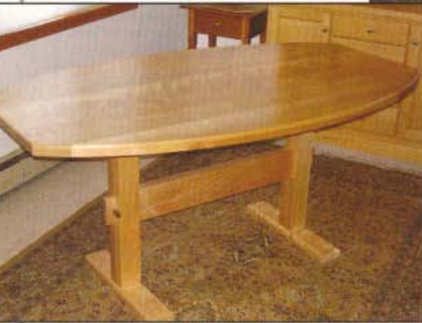
Rounded edges — This trestle-style dining room table, with rounded edges to maximize the people it could seat, was made from yellow birch. The top was cut out on the Multi-Cam CNC router, with very little sanding required.
