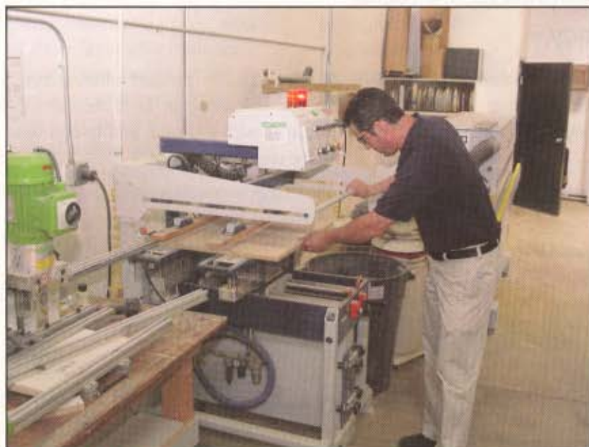
Twice as efficient — Vargo says the Toola double line boring machine saves time and prevents mistakes that were common with the previous equipment.
