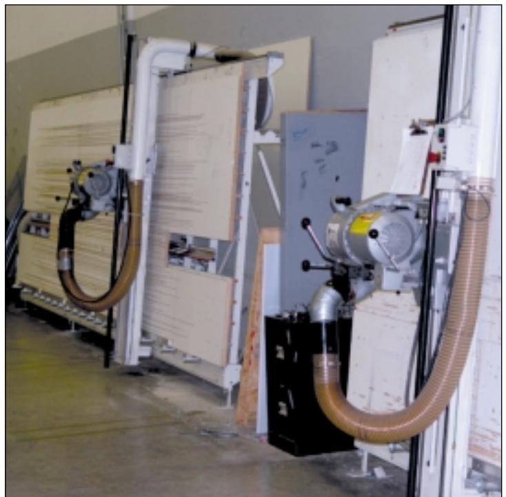
These two Striebig Vertical Panel Saws have helped Karas & Karas become the leading fabricator/installer of ACM panels in New England
