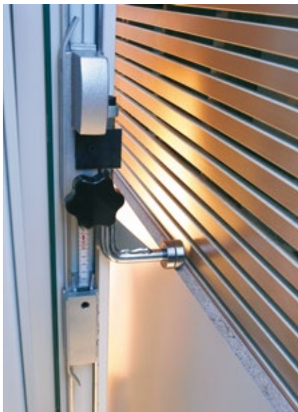
The standard strip cutting gauge with edge-protecting roller support makes repeat cuts easier.
